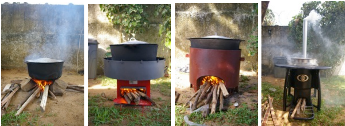
Fig. 21: Three-stone fire (baseline), Prakti’s “Orka”, “Kala” stove, Envirofit “EFI 1001” (from left to right)
