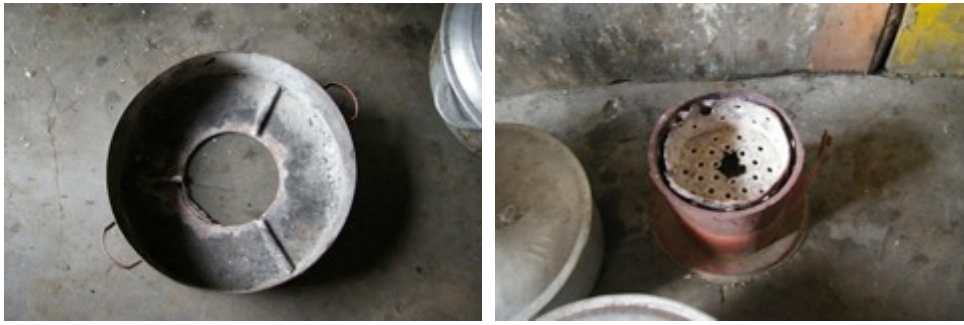
Fig. 13: The XL RFP at Aquila Restaurant showed damages after one year of heavy everyday use. Besides the broken seat, the stove (new design) showed that the rim of the inner cylinder is corroded while the 1.5mm top part is still in good condition.
