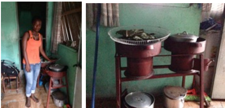
Fig. 12: During the household visit at Olive Kun, I found the two RFPs in a good condition, even though the stoves are done with the old design. She is using the stoves everyday since June 2014 and carefully maintaining them. She even went to a welding shop to repair the top part.
