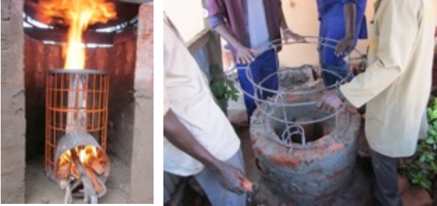
Fig. 27: Combustion chamber by Rocket Works (left), outer brick structure and metal pot rests (right), Christa Roth, 10/15
